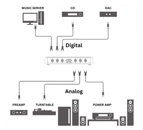
You may use one side for Digital equipment, and another side for Analog. Terminals 1, 2, and 3 are recommended for connecting digital devices, while terminals 4, 5, and 6 are recommended for connecting analog devices. Or you can simply use two Foundation Ground Core to separate digital and analog equipments.
